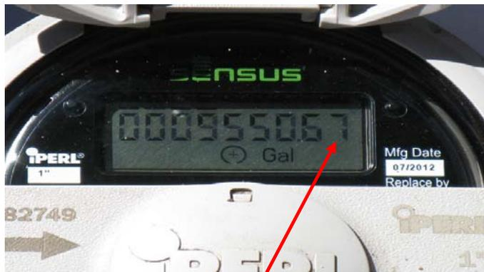
**Leak Detection - Far Right Digit = 1/100th of gallon of water
