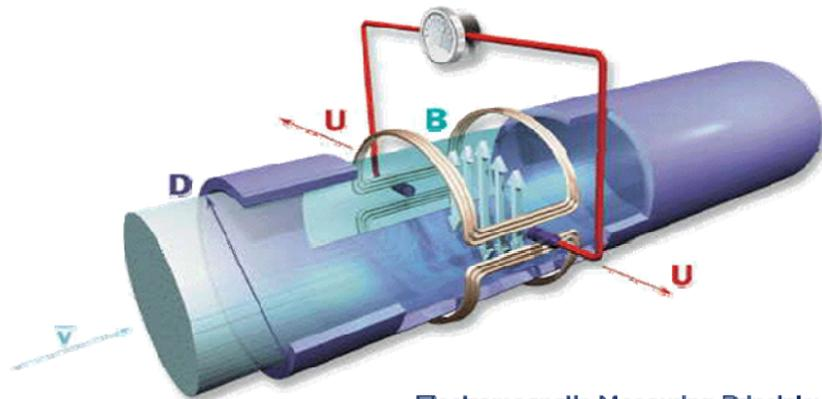
**Electromagnetic Measuring Principle:**
